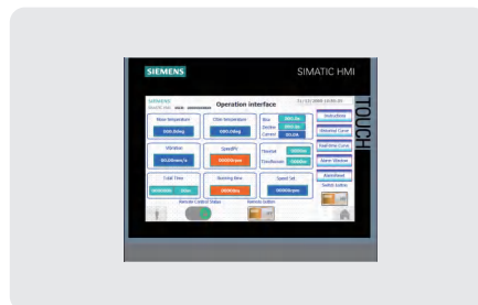
Touch Screen Control System (Siemens PLC)
